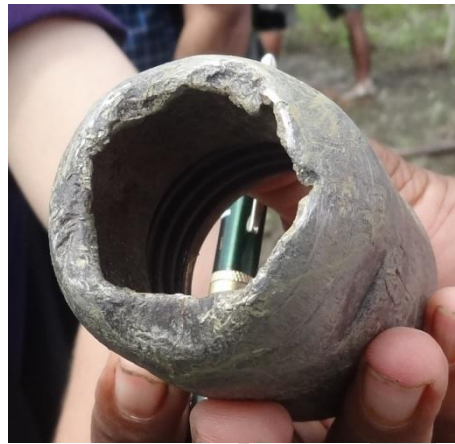
Fig. 2. SPT Sampler Shoe with Blunt Bottom used in the SP Tests
