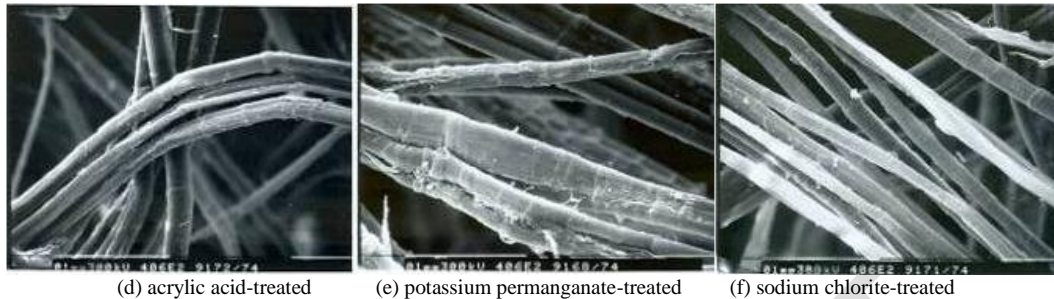
Fig. 3: Scanning electronic micrographs of flax fibre surface after different surface modifications
