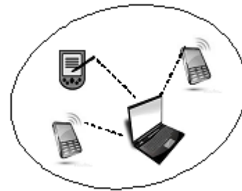
Figure 2: Piconet with one master and three Slaves
