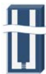
Figure 1: Silicon substrate with platinum electrodes
