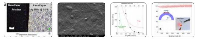
Figure 1: Optical view of (A) Nanopaper substrate before and after the deposition of Ag Nws. B) Sem image of a tin coating sputtered onto nanopaper. (C) Square resistance of nanopaper and PET substrates as function of Ag NWs density and TiN deposition time. (D) Square resistance of a TiN coated nanopaper after 650 mechanical bending. The inset show the bending principle.
