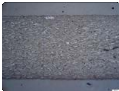
Figure 1: Fiber orientation and distribution in the neck region of a sintered (at 1250 °C) tensile specimen.
